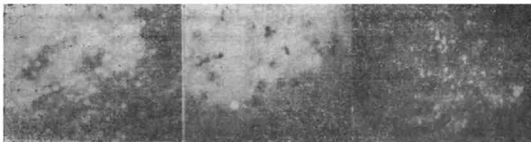
Fig 2. Microphotograph of voids produced in steel by 1 MeV electron irradiation under low dose influence at 550℃ (a) 316 steel, 8 dpa, \times 20 K (b) 316 steel bearing 1%Si, 7.3 dpa, \times 20 K (c) 316 steel bearing 0.1%Ti, 7.3 dpa, \times 20 K
