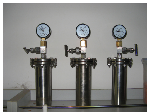
Fig.2 The designed photo of the airproof container for gas collection
